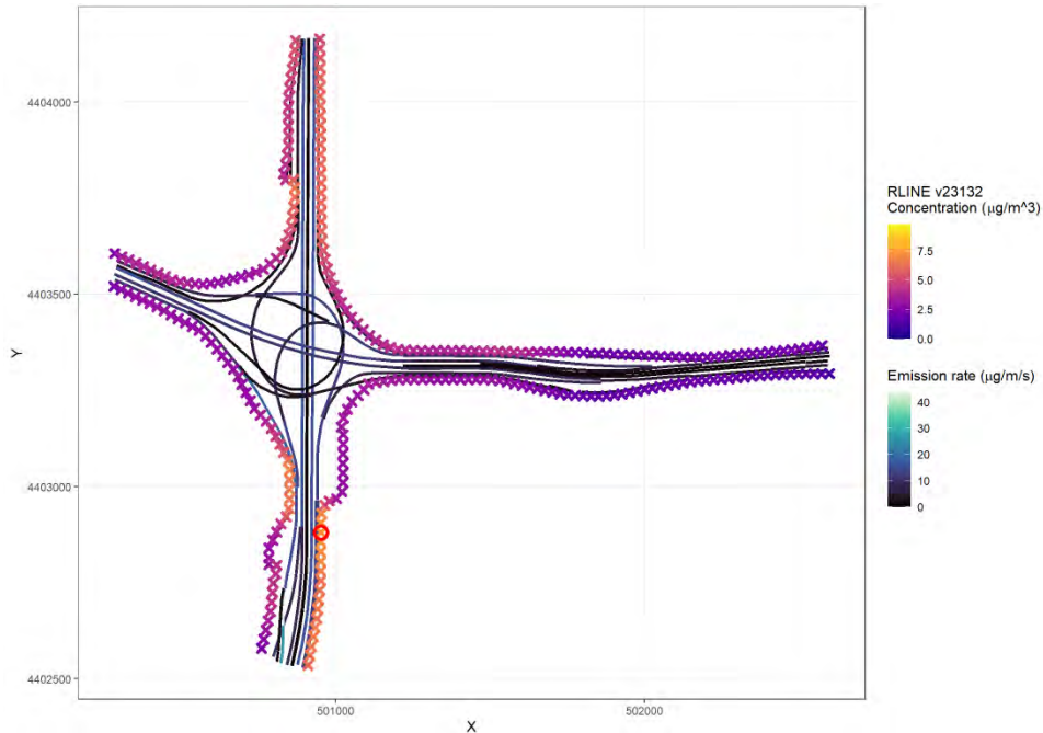
Figure 13 Project layout for the Project A hot spot analysis. RLINE emission source drawn as lines with emission rate shaded (black - blue - green). Receptor locations indicated with X's and RLINE v23132 model concentrations shaded (purple - yellow). Design concentration receptor location indicated with red circle.
