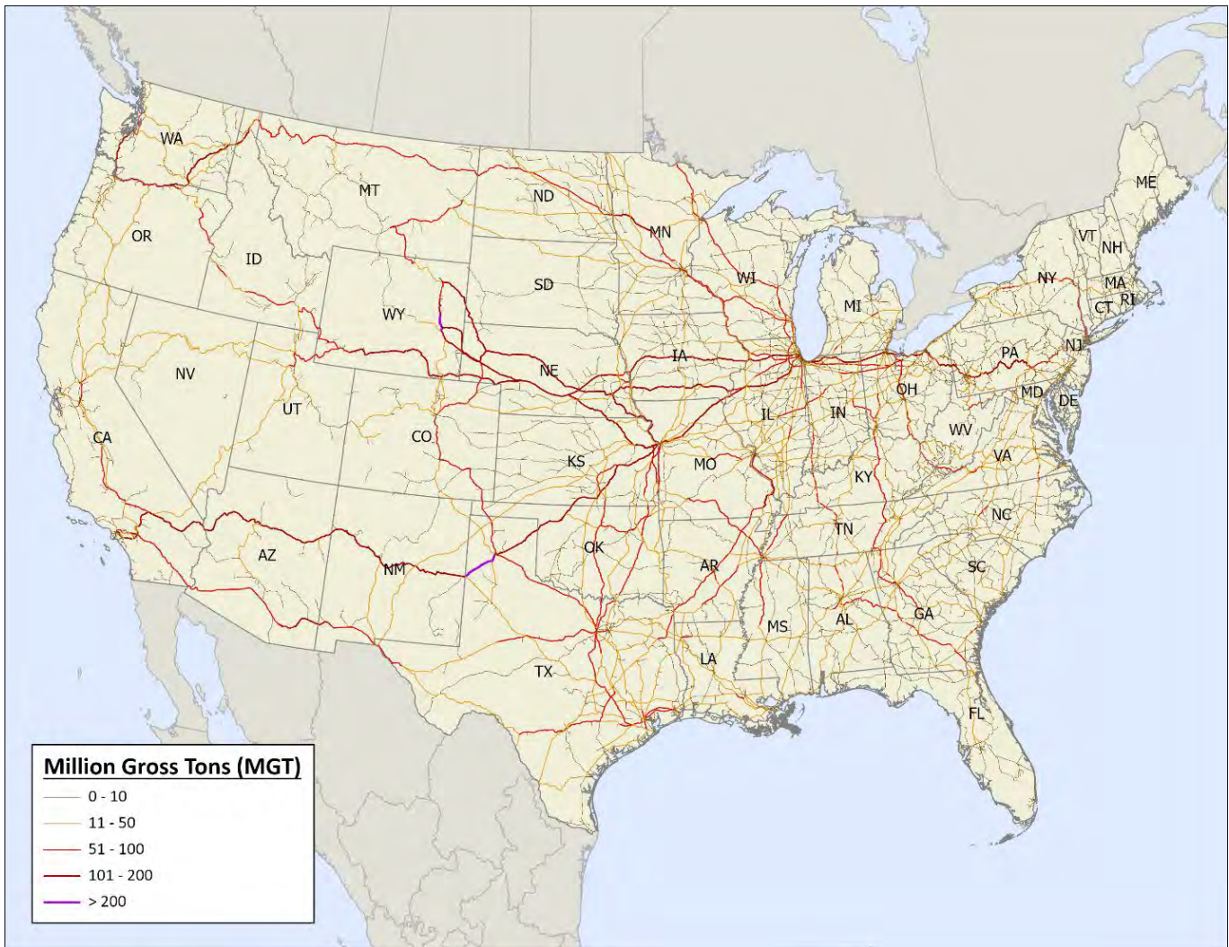
Figure 2-5. 2017 US Railroad Traffic Density in Millions of Gross Tons per Route Mile (MGT)
